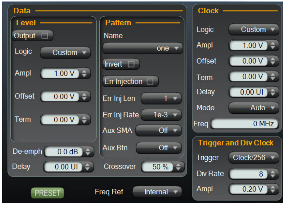
Figure 37. N4971A control panel
