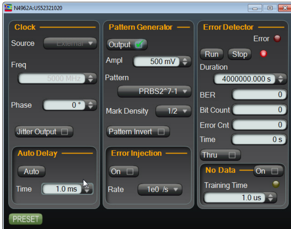
Figure 43. N4962A control panel
