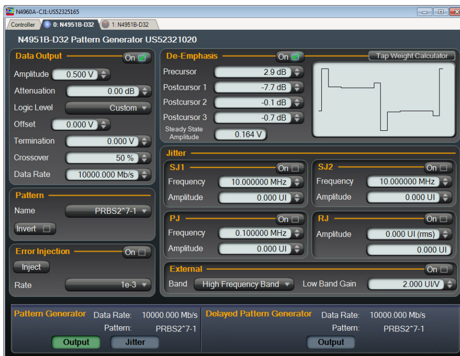
Figure 110. Access pattern generator control panel
